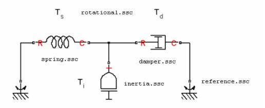
The domain is declared in a file named rotational.ssc (see "Example — Declaring a Mechanical Rotational Domain" on page 2-12). The following file, named spring.ssc, declares a component called spring. The component contains:
