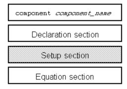
The setup section of a Simscape file follows the declaration section and consists of the function named setup. The setup function is executed once for each component instance during model compilation. It takes no arguments and returns no arguments.
